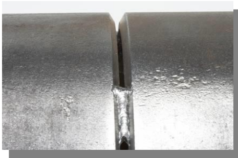
Steel Pipe – Tack Welded
